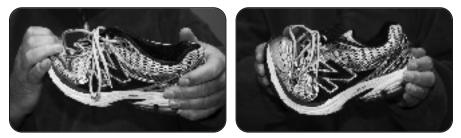
**Twist Test** – Hold heel firmly in left/right hand and try to rotate the tow back and forth; you should not be able to fully turn the shoe and it should "bounce back".
